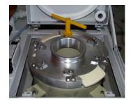
Re-install the rotor, secure the lock catches, close the housing cover and switch on the centrifuge.
