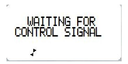
The screen below is displayed when the system detects no flow through the electrolytic cell housing. This condition will stop the system from generating chorine. Once flow is restored, the system will start automatically and this screen will no longer be active.
