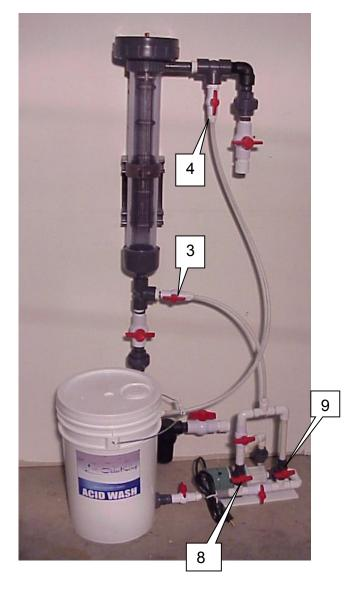
Plug the Acid Wash pump in to a 120 VAC source and start the wash cycle. Allow the pump to run until the cell is clean.
