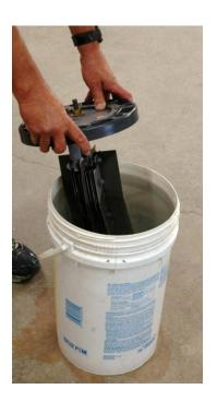
Clean the cell when calcium buildup is present with the ChlorKing® Acid Wash System (non-reverse polarity system)
