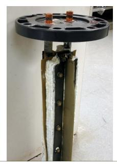
A cell stack with calcium bridged plates.
